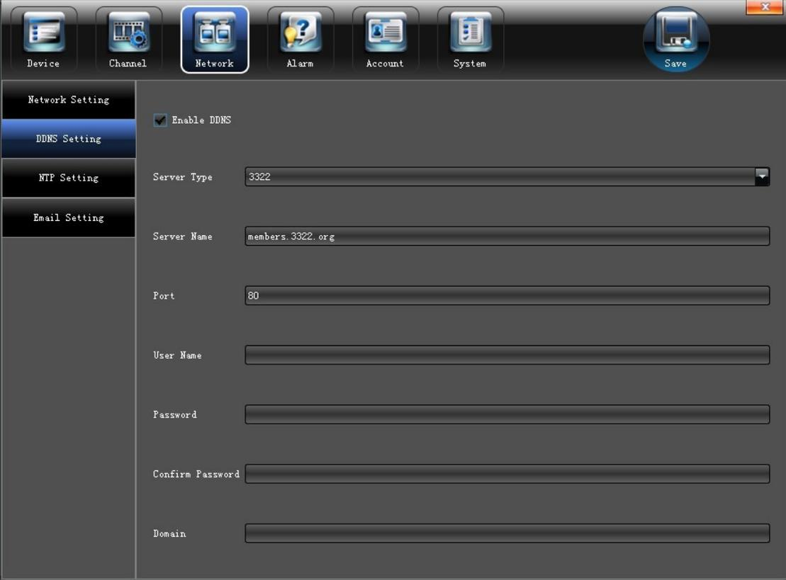
The screenshot shows a web-based configuration interface for a device. At the top, there is a navigation bar with icons for Device, Channel, Network, Alarm, Account, System, and a Save button. The 'Network' icon is highlighted. Below the navigation bar, there is a sidebar with menu items: Network Setting, DDNS Setting (highlighted), NTP Setting, and Email Setting. The main content area is titled 'Network Setting' and contains the following fields:
